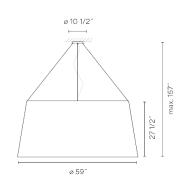
Electrical characteristics 5 x A-19 LED LAMP 120V 8W
