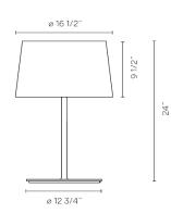
Electrical characteristics 3 x A-19 LED LAMP 120V 8W
