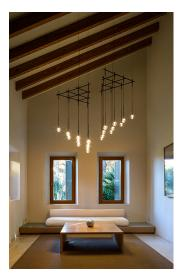
Light source: 2700K CRI >80 3122 Im 99 Im/W Fixture: 1545 Im 49 Im/W Driver included: CC - Constant Current 1050 mA 120~277V 50/60Hz
