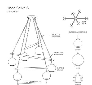
Upper Crossbar: 36", Middle Crossbar: 48", Lower Crossbar: 24" Crossbar length is from center to center of glass shade Total Horizontal and Vertical dimensions of fixture depend on glass shade selection Materials: glass, metal, wood Total Product Weight: with 6.5" Orb: 30 lbs; with 9.0" Orb: 36 lbs; with 7.0" Urchin: 30 lbs
