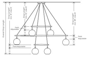
\* Drop length measured from ceiling to crossbar. 6.5" Orb and 9" crossbar to crossbar distance shown.
