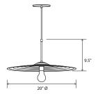
Dimensions: 20" Ø, 9.5" Materials: solid brass Product weight: 6 lb Light source: medium base E26 socket Lamping: 1x E26 base, 60 W max Bulbs not included Input voltage: 250 V AC max Textured Black Powdercoat (CM-049) low profile round canopy with Black Cloth Covered Cord (CM-090) Canopy dimensions: 5" Ø, 0.3" See website for more canopy information Field adjustable drop length: 0'9" min - 8'0" max Suitable for a sloped ceiling Specifications subject to change
