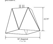
Dimensions: 25" x 25", 22.75" Materials: wood, metal, polymer Product weight: 18 lb Light source: 4x GU-24 base socket Lamping: 4x GU-24 base, 18 W max each Bulbs not included Input voltage: 300 V AC max White (CM-060) 8" round canopy included Canopy dimensions: 8"Ø, 1.25" See page left and website for more canopy information 96" drop length, field adjustable Suitable for a sloped ceiling Wood grain will vary Specifications subject to change
