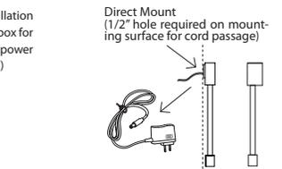
\* Hardwired installation requires room in the j-box for the included external power adapter (2" x 1" x 1.25")
